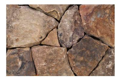
GEOLOGY: SANDSTONE THICKNESS: 0.75"-1.75" SIZE RANGE: 6"-18"DIAMETER WEIGHT: TYPICALLY 13 LBS./SQ. FT. DENSITY (ASTM C97): 156 LBS. /CU. FT. ABSORPTION (ASTM C97): 1.9% COMPRESSIVE STRENGTH (ASTM C170): 16,550 PSI FLEXURAL STRENGTH (ASTM C880): 1,580 PSI
